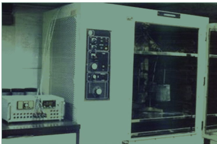
Fig. 1. Photograph and diagram of the isothermal oven employed.
